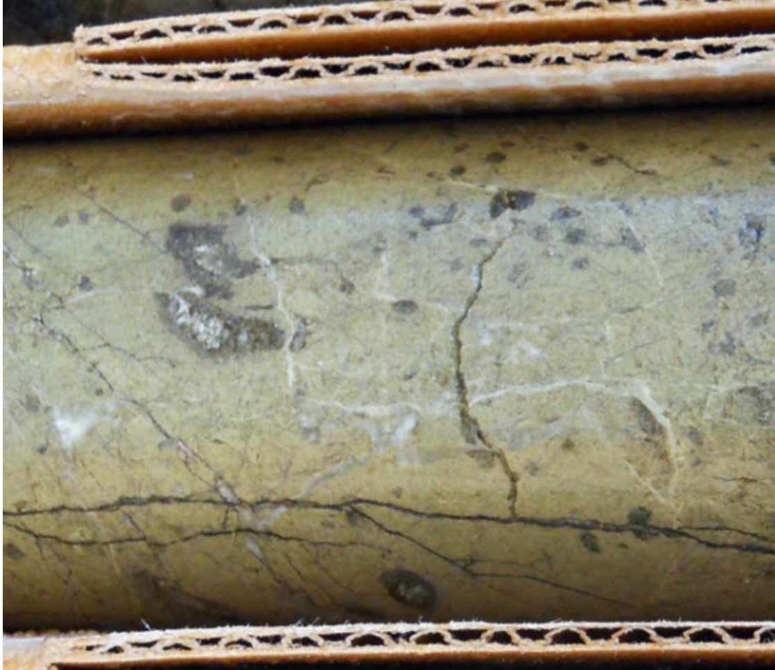
Greenish colored propylitic alteration with calcite veining in andesitic volcanics at the Rosemont deposit, Pima County, Arizona (Photo taken January 2012, September 2012).
