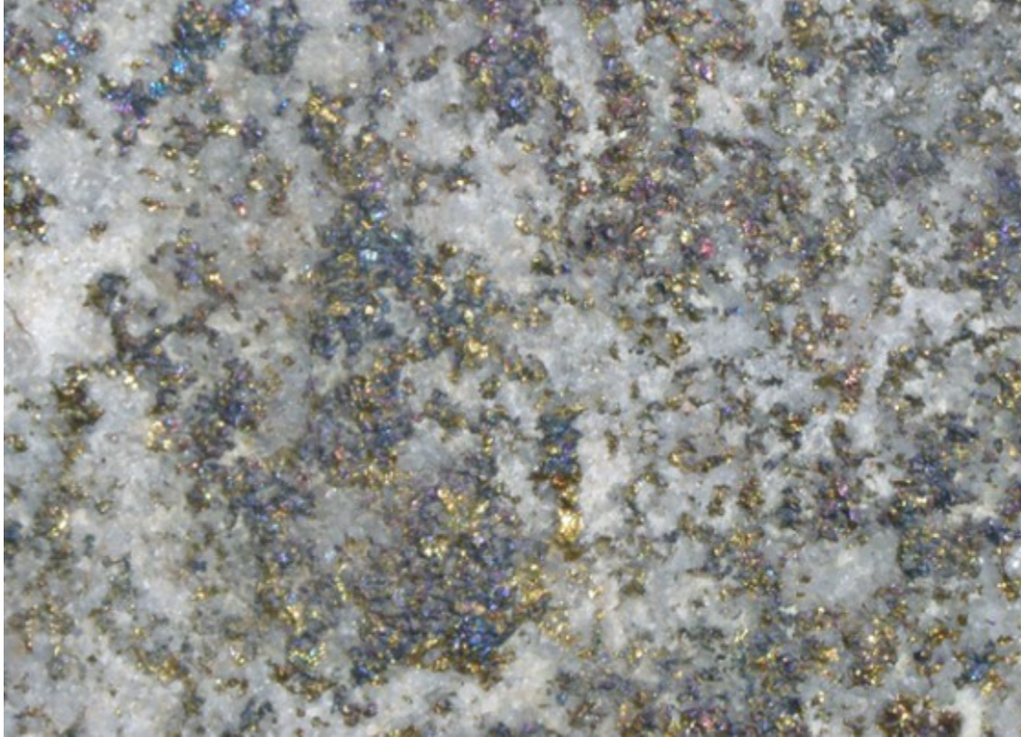
Chalcopyrite-Bornite-Quartz Vein from Freeport's Dos Pobres mine near Safford, Arizona (Photo taken by David Briggs)
