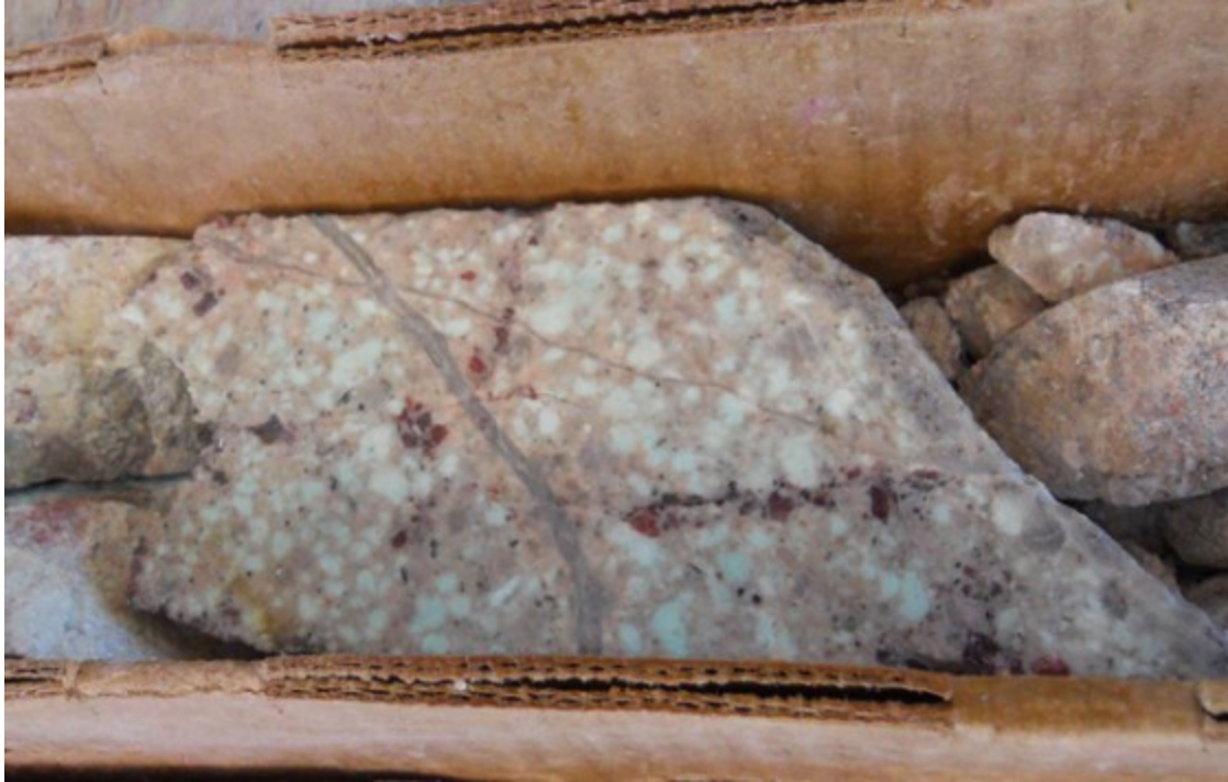
Porphyry with feldspar and quartz phenocrysts and quartz veining. This 4-inch long sample is from the Rosemont deposit, Pima County, Arizona (Photo taken by Jan Rasmussen, September 2012).
