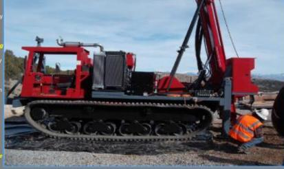
The R-40 was custom designed to fulfill this need: it is mounted on a rubber track carrier that allows the R-40 to minimize environmental disturbance, while the robust design and modern hydraulics allow the rig to drill to depths that would normally require much larger and heavier rigs: the R-40 however, remains as economical as a much smaller drill and can be used for shallow hale drilling.
