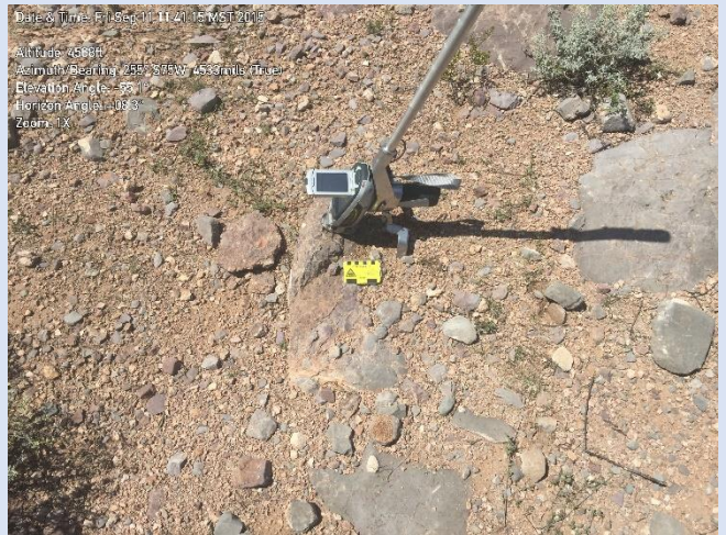
19. Niton geochem on Breccia pipe Sept. 2015
