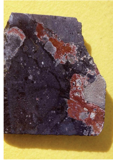
Figure 17. Oxidized/reduced breccia with uraninite and hematite. FOV=4in. Pinenut Mine
