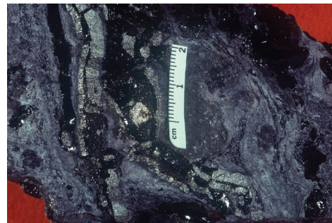
Figure 31. Bitumen formed after most stages of mineralization and fracturing. Note the fractured pyrite, but unfractured bitumen. The bitumen is only known to occur in significant concentrations in 2 of the mineralized breccia pipes
