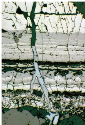
Figure 21. Alternating bands of siegenite, pyrite, & bravoite cut by a later vein of galena. Pigeon Mine. Field of View = 0.9mm
