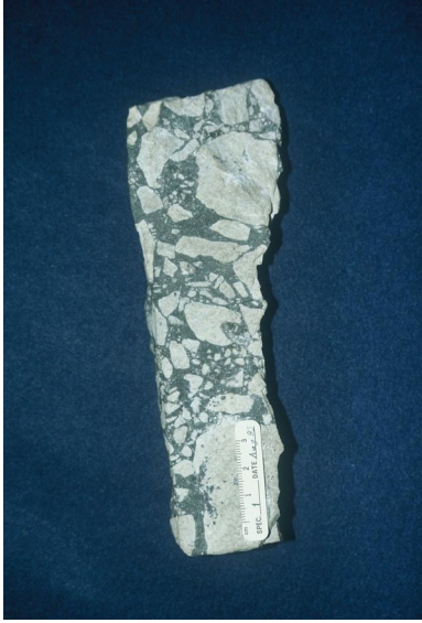
Figure 4. Core from Hack 2 breccia pipe. Sandstone, limestone, & shale clasts in a polymetallic uraninite matrix.
