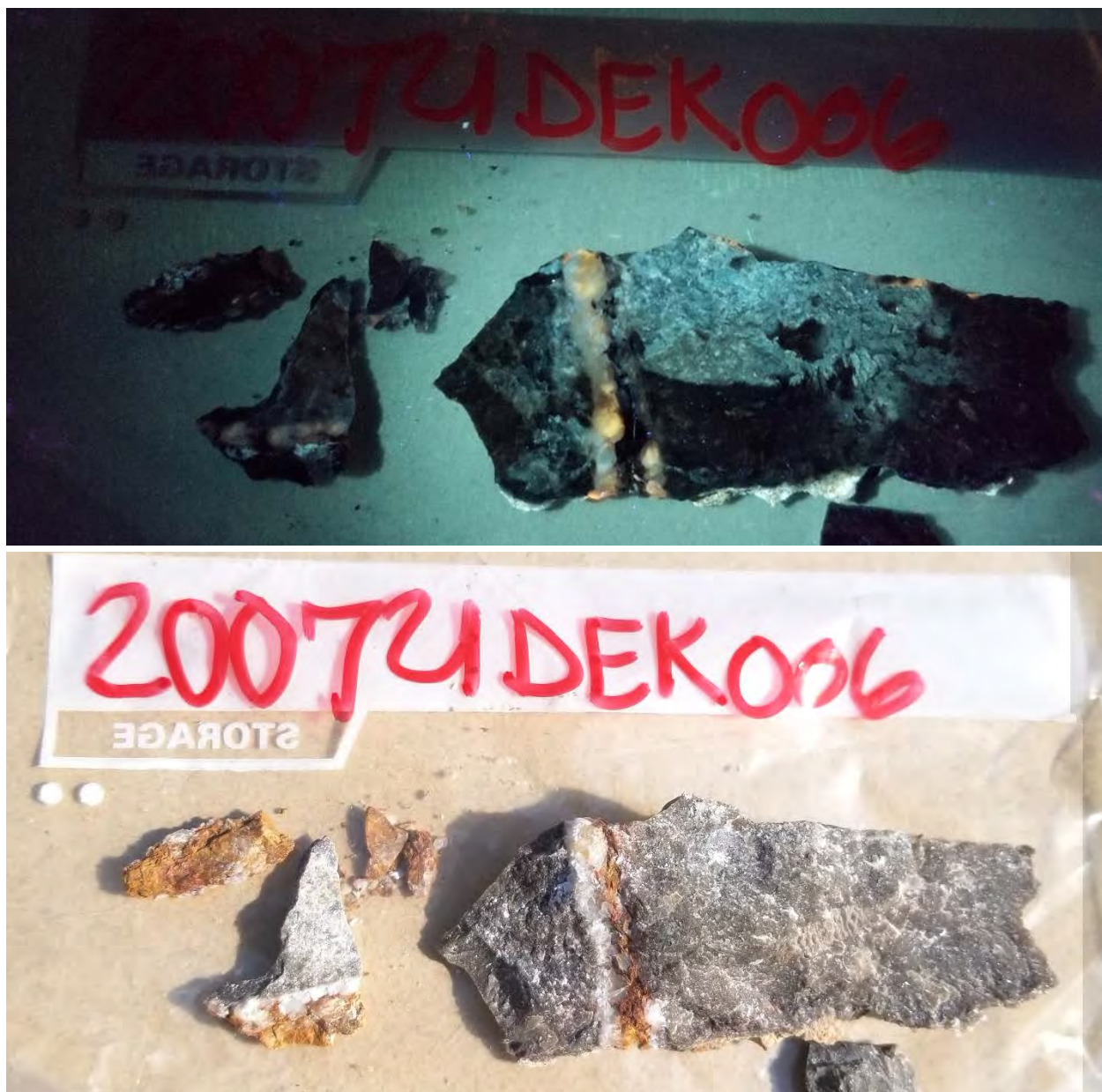
Figure 55: Type 1 vein showing orange UVF. Top photo is under UV light bottom photo is under daylight.
