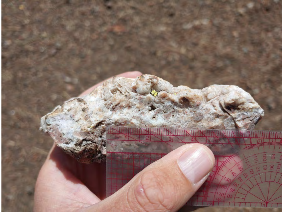
Figure 47: Hand sample from structurally controlled breccia crosscutting Tertiary rhyolite from the Rhyolite Hills
