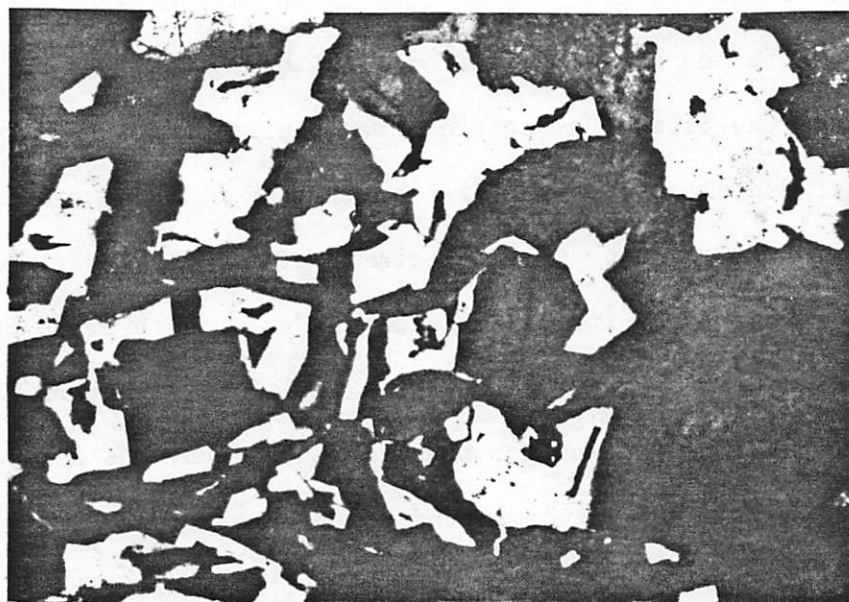
Fig. 7.--Photomicrograph of the granophyre, showing a micrographic texture with cuneiform intergrowths of quartz and argillized orthoclase (48X, crossed nicols).
